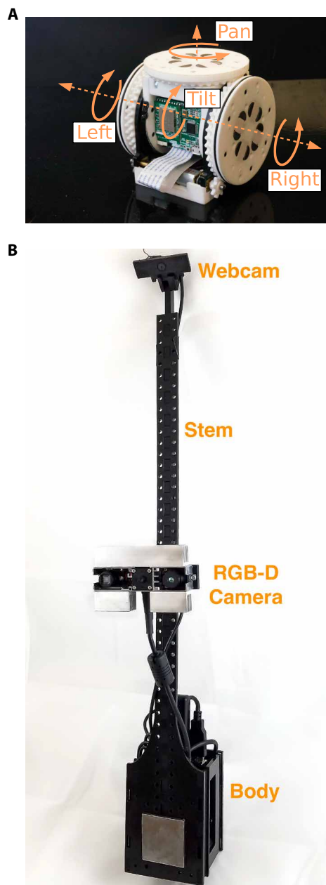
Fig. 4. SMORES-EP module and sensor module. (A) SMORES-EP module. (B) Sensor module with labeled components. UP board and battery are inside the body.
