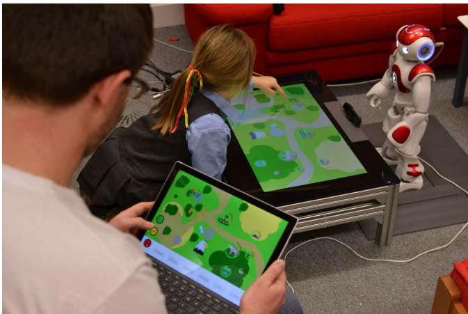
Fig. 2. Setup used in the study. A child interacts with the robot tutor with a large touchscreen sitting between them, displaying the learning activity; a human teacher provides guidance to the robot through a tablet and monitors the robot's learning. Although the picture depicts an early laboratory pilot, the main study was conducted on actual school premises.
