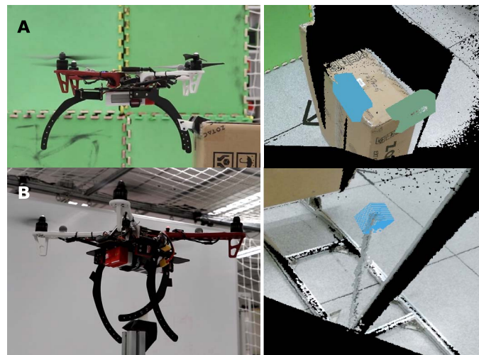
Fig. 4. Example resting actions with vision-based perching and resting location detection. (A) Resting on a box's edge ( R_e ). (B) Stand-resting on a stick ( R_s ).
