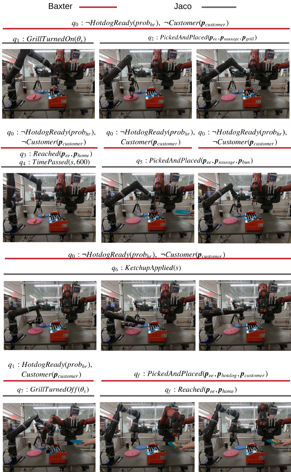
Fig. 3. Example execution trace of the hot dog cooking and serving task. Each snapshot represents a change in the FSPA (change of a predicate truth value and/or transition on the FSPA). The gray and red paths trace the steps necessary to trigger a transition on the FSPA (for either robot) shown in Fig. 2 (A and B). The FSPA state along with the corresponding edge guard is provided on top of each path.
