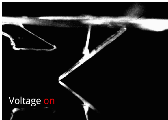
Movie 2. Video taken with a high-speed camera showing the DEAnsect movement slowed down by 140 \times . The side view of the DEAnsect body and leg shows the motion principle.
