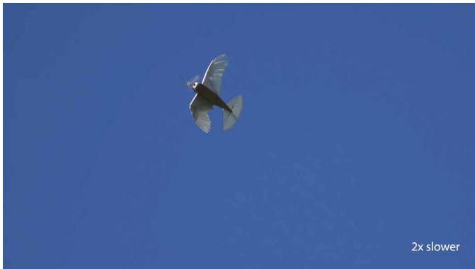
Movie 3. PigeonBot untethered flight responses to wing asymmetry. With PigeonBot flying straight and level, we commanded wing asymmetries while locking the rudder neutral and measured the resulting kinematics. Feathered wing asymmetry causes primarily roll with adverse yaw.
