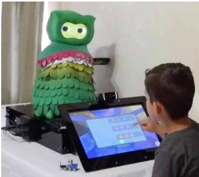
Fig. 1. Long-term, real-world SAR intervention setup. In this month-long, in-home study, child participants with ASD played math games on a touchscreen tablet, while a socially assistive robot used multimodal data to provide personalized feedback and instruction (37).
