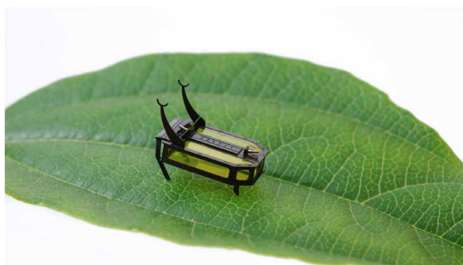
Movie 1. RoBeetle, an 88-mg autonomous robotic insect powered by fuel. Summary of results and methods.
