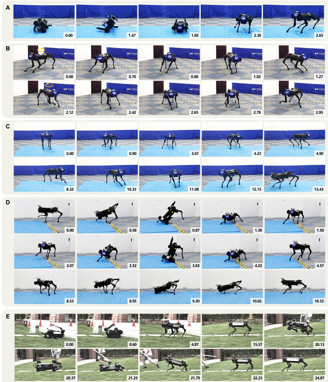
Fig. 5. Dynamically synthesized MELA policy running on a real quadruped robot and demonstrating adaptive and agile locomotion behaviors. (A) Successful fall recovery performed by the MELA expert, inheriting original skills from the pretrained experts. (B) Newly emerged skills, dynamic steering on the spot, naturally learned through the MELA framework. (C) Target-following experiment with simultaneous trotting and steering using online synthesized skills. (D) Target-following experiment showing the capability of failure-resilient trotting and critical recovery within one second (average of 0.5 s for restoring body posture and 0.4 s for returning to the trotting mode). (E) Adaptive trotting and fall recovery experiment on a sloped grass field, showing the capability of robust traversal in an unstructured environment. Time in snapshots is measured in seconds.
