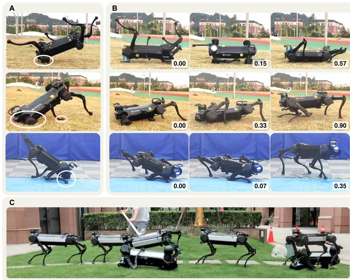
Fig. 1. Challenging locomotion scenarios and agile maneuvers of a quadruped robot. (A) Three challenging scenarios of the Jeuying robot during various tests: unexpected body contacts with the environment and unpredictable robot states. The white circled regions highlight unusual contact that can occur at any part of the body. (B) Different adaptive behaviors from our proposed learning framework that generated dynamic motions and complex coordination of legs for immediate recovery from failures. Time in snapshots is measured in seconds. (C) Resilient locomotion using adaptive skills in the presence of unexpected disturbances.
