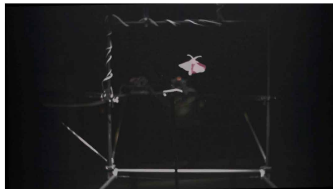
Movie 2. Tracking A. ipsilon moths with extraction of flight kinematics by 3D model-based matching (real moth in white and 3D model in pink).
