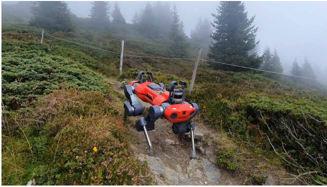
Movie 1. Robot in the wild. A learning-based locomotion controller enables a quadrupedal ANYmal robot to traverse challenging natural environments.
