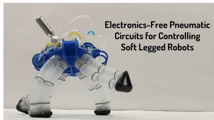
Movie 1. Electronics-free air-powered circuits to control the rhythmic movement of a soft legged robot.
