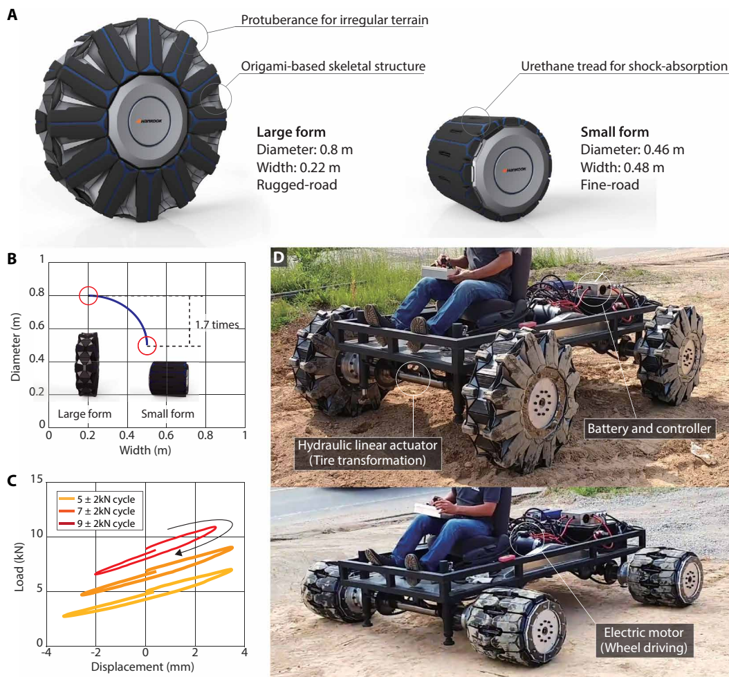
Fig. 1. Transformable wheel concept and demonstration. (A) The wheel can be transformed into two shapes according to the road condition. (B) The relationship between the diameter and width of the wheel. (C) The load-displacement response of the wheel in the shape-transition state. (D) We designed a single-passenger vehicle for installation of the transformable wheels. The operation and capacity of the wheels were demonstrated through a field test.
