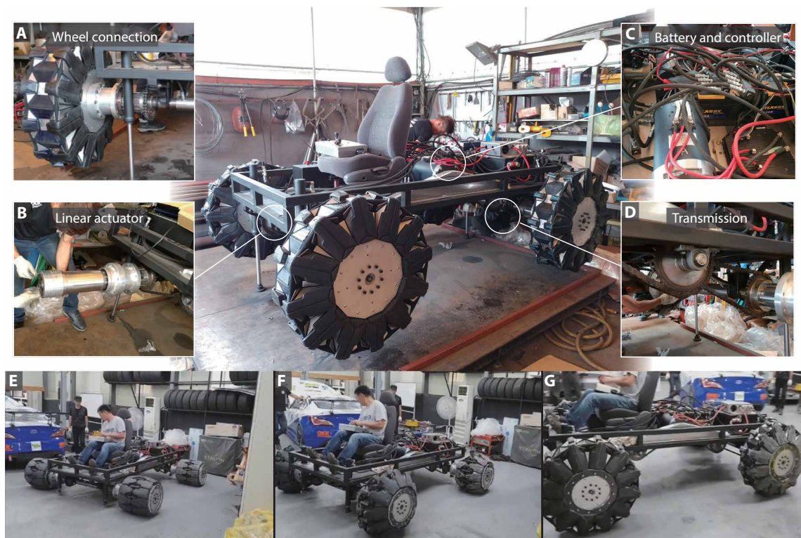
Fig. 6. Vehicle implementation and field test. (A) The wheel connection is designed for independent control of driving (wheel rotation) and transformation (wheel hub translation). (B) A hydraulic pressure system enables transformation. (C) The vehicle uses two electric motors for driving, and (D) the driving torque is transmitted through a chain. (E to G) On-site verification of wheel transformation, which can also be performed while driving.
