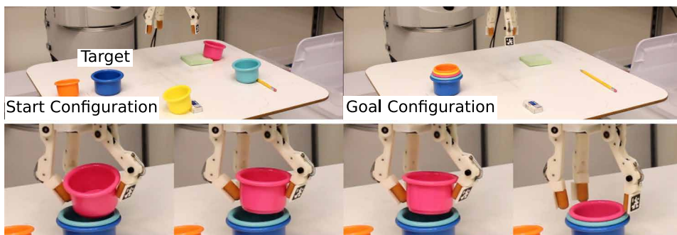
Fig. 7. A cup-stacking task requiring the hand to align both the position and the orientation of cups. The hand was installed on an arm; the task was to pick up all cups from the table and stack them into the target blue cup. At the bottom of each cup, there was an AprilTag for the in-hand camera to observe the POM.
