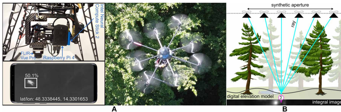
Fig. 1. Autonomous drone supporting SAR missions. (A) Camera drone with the recording and processing equipment used in our experiments. In the case of a positive finding, an integral thermal image from the AOS approach, together with classification result and location are transmitted to a mobile device of the rescue team. (B) Basic principle of AOS. Movie S1 shows a video footage of the drone and sample test site.
