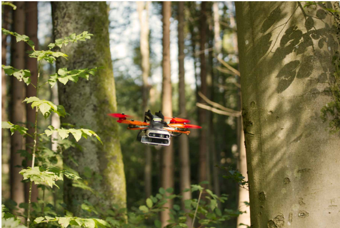
Movie 1. Demonstrations of agile flight in challenging environments with purely onboard sensing and computation. The video also summarizes the training methodology of the navigation policy.
