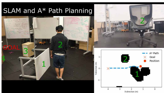
Movie 4. Demonstration of the Augmented Cane performing closed-loop planning to navigate to a desired indoor position in a cluttered environment. The Augmented Cane used LIDAR-based SLAM to determine the position of the participant and the environment. This map was then filtered to detect obstacles, and a path planning algorithm, A^* , computed a trajectory to safely reach the desired position. The grounded kinesthetic feedback then steered the user along this trajectory.
