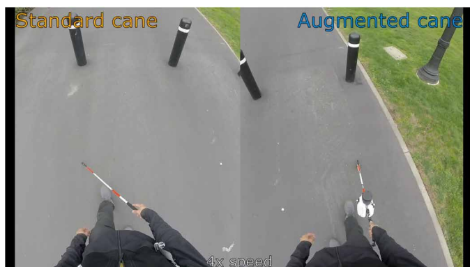
Movie 3. Comparison of the Augmented Cane and a white cane during an outdoor experiment. A time lapse of a novice participant navigating an outdoor asphalt path with the Augmented Cane and a white cane with audio feedback.
