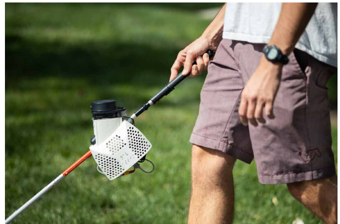
Movie 1. Summary of the Augmented Cane. The Augmented Cane uses a multimodal set of sensors to perceive the environment and provides grounded kinesthetic feedback to steer the participant. A series of experiments evaluated how novice and expert participants navigated when using the Augmented Cane or a white cane.
