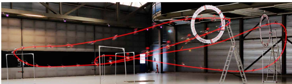
Fig. 1. A time-optimal trajectory. This time-optimal flight path was computed using the proposed CPCs and executed in a motion capture system, outperforming the best human expert.
