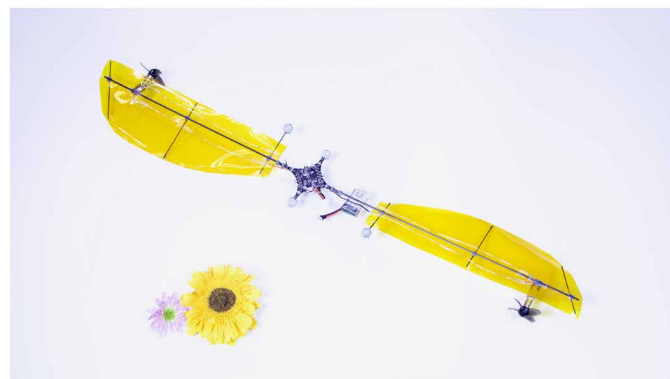
Movie 1. Overview of the bioinspired revolving-wing drone.
