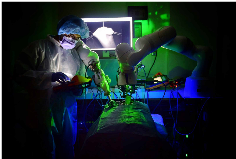
Movie 1. Overview of the Smart Tissue Autonomous Robot (STAR) for autonomous laparoscopic soft tissue anastomosis.
