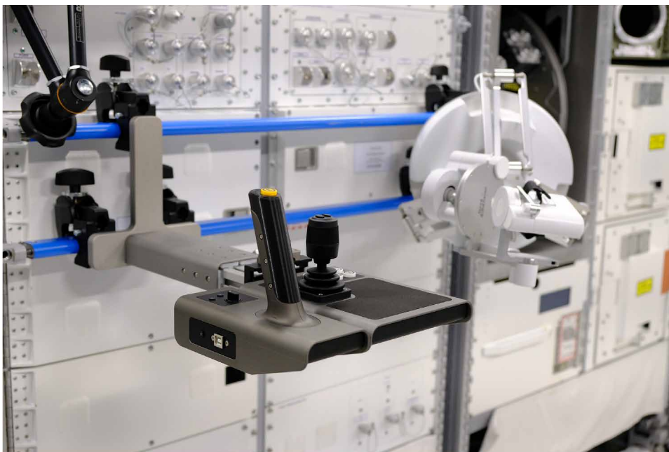
Fig. 7. Close-up view on the setup aboard the ISS. Space-qualified haptic interfaces on the ISS including the FF device sigma.7 and the custom-built joystick.
