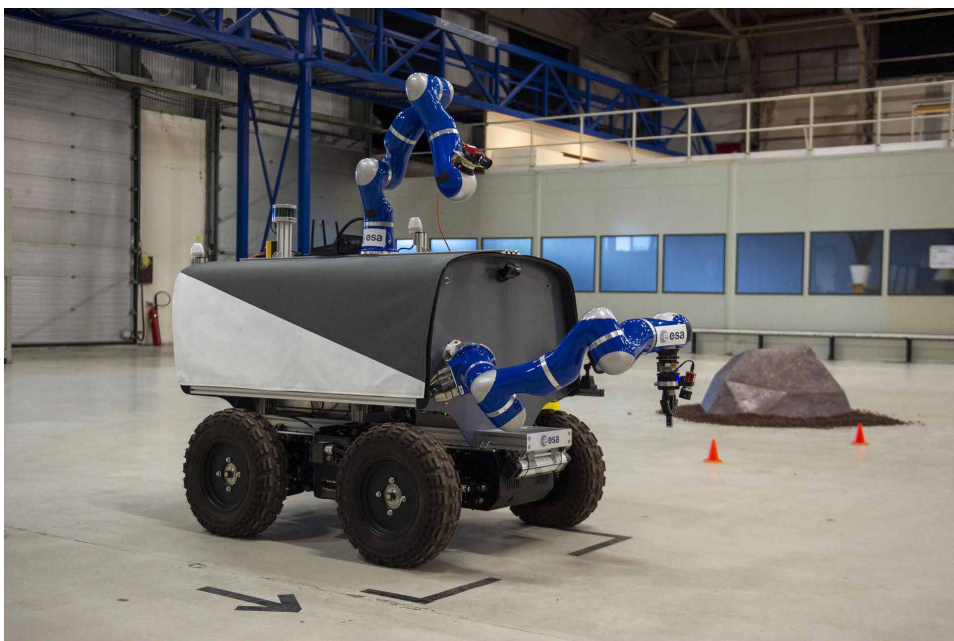
Fig. 8. On-ground setup. The all-terrain, four-wheel drive rover with two robotic manipulators for sample picking and head camera motion, respectively.
