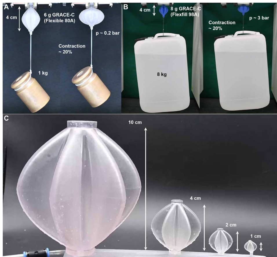
Fig. 2. GRACE muscles with tunable force output and scalable size. (A) A 4-cm-long, 6-g GRACE made of Flexible 80A resin by Formlabs (SLA) lifts up a 1-kg load with a contraction of 20% lengthwise. (B) A 4-cm-long, 8-g GRACE made of Flexfill TPU 98A by Fillamentum (FDM) lifts up an 8-kg load with a contraction of 20% lengthwise. (C) GRACEs of sizes spanning one order of magnitude.
