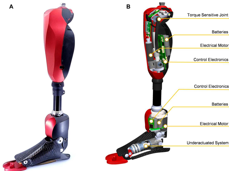
Fig. 1. System overview. (A) A photo of the Utah Bionic Leg. (B) Partially sectioned view of the prosthesis model highlighting the main electrical and mechanical components.
