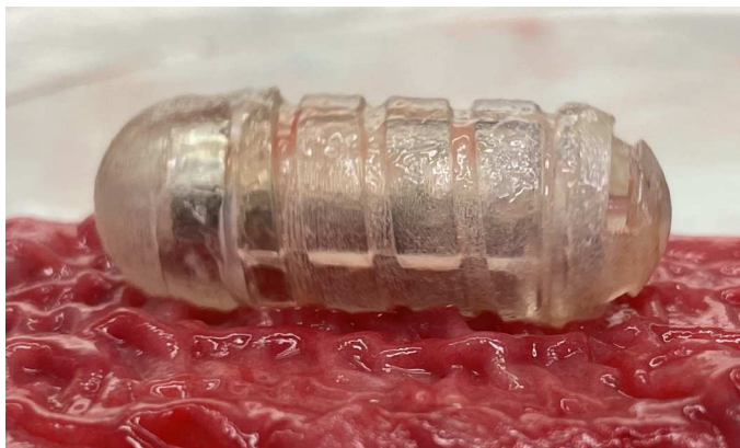
Movie 1. Overview of the RoboCap: The RoboCap is an ingestible capsule that robotically clears intestinal mucus and delivers drugs to heighten absorption and bioavailability.
