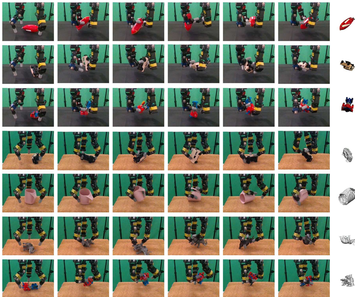
Fig. 5. Reorientation of real objects. Examples of reorienting real objects that were not 3D printed using a four-fingered and a three-fingered manipulator.
