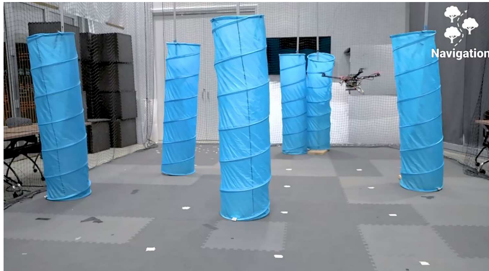
Movie 1. Demonstration of real-world quadrotor experiments using uncertainty estimation in optical flow.
