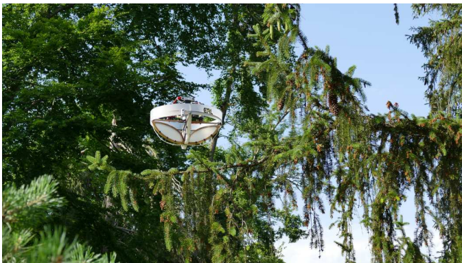
Movie 1. Collecting eDNA with the eDrone. The drone combines a haptic-based control strategy with a protective cage to land on tree branches. Surface eDNA is then collected using an adhesive surface integrated into the cage.
