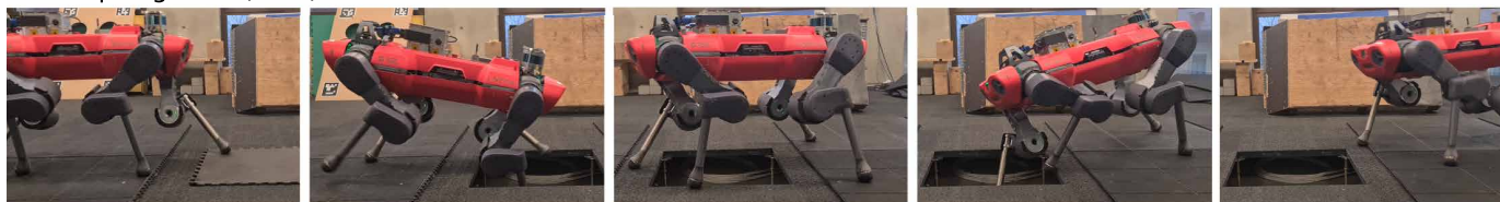
Fig. 4. Benchmarking against model-based control. (A) DTC successfully traverses an obstacle parkour (left to right) in simulation with a heading velocity of 1 m/s. (B) Baseline-to-1 falls after stepping into a gap hidden from the perception (left to right). (C) ANYmal successfully overcomes a trapped floor using our hybrid control architecture (left to right).
