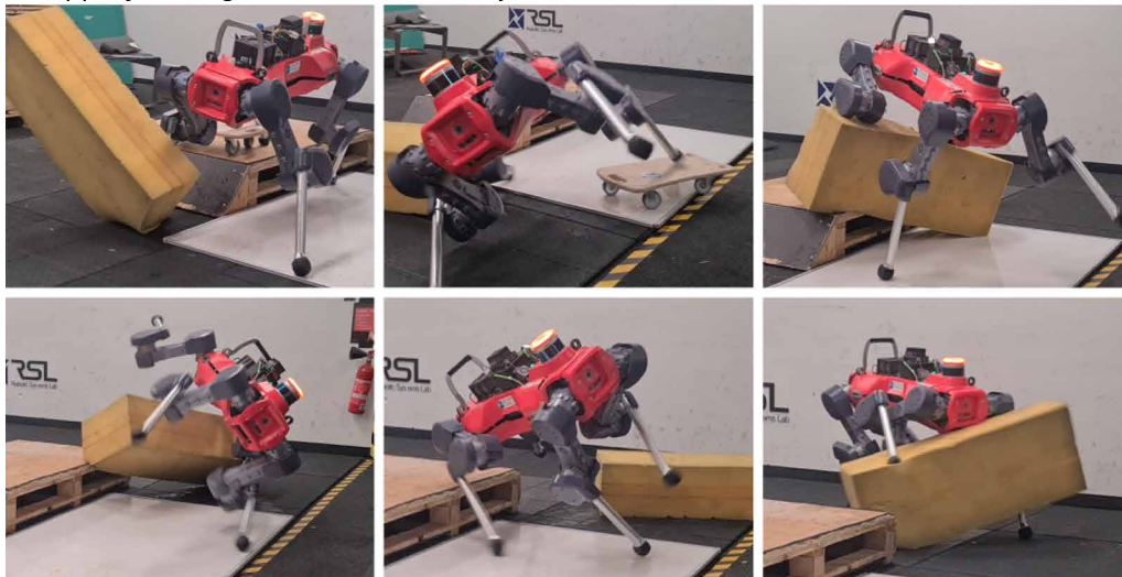
Fig. 2. Evaluation of robustness. (A) ANYmal walks along a loose cover plate that eventually pitches forward (left to right, top to bottom). The third row shows ANYmal's perception of the surroundings during the transition and recovery phase. (B) The snapshots were taken at critical time instances when walking on slippery ground, just before complete recovery. (C) ANYmal climbs up stairs with disabled perception (top to bottom). The collision of the right-front end effector with the stair tread triggers a swing reflex, visualized in orange.
