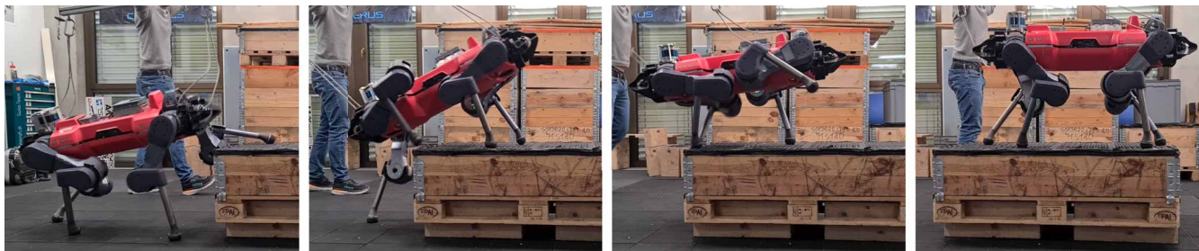
Fig. 3. Evaluation of tracking performance. (A) ANYmal climbs up a narrow table, turns, and descends back down to a box. The second image in the second row shows the robot's perception of the environment. (B) Euclidean norm of the planar foothold error, averaged over 20 s of operation using a constant heading velocity. The solid/dashed curves represent the average/maximum tracking errors. (C) Same representation as in (B), but the data were collected with baseline-to-2. (D) DTC deployed with baseline-to-2, enabling ANYmal to climb up a box of 0.48 m.
