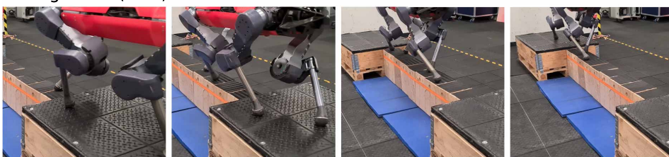
Fig. 5. Benchmarking against reinforcement learning. (A) Baseline-rl-1 attempts to cross a small gap. ANYmal initially manages to recover from miss-stepping with its front legs but subsequently gets stuck when its hind legs fall inside the gap. (B) Using baseline-rl-1, the robot stumbles along a narrow beam. (C) With DTC, the robot can pass four consecutive large gaps (left to right) without getting stuck or falling. (D) ANYmal is crossing a long beam using the proposed control framework.
