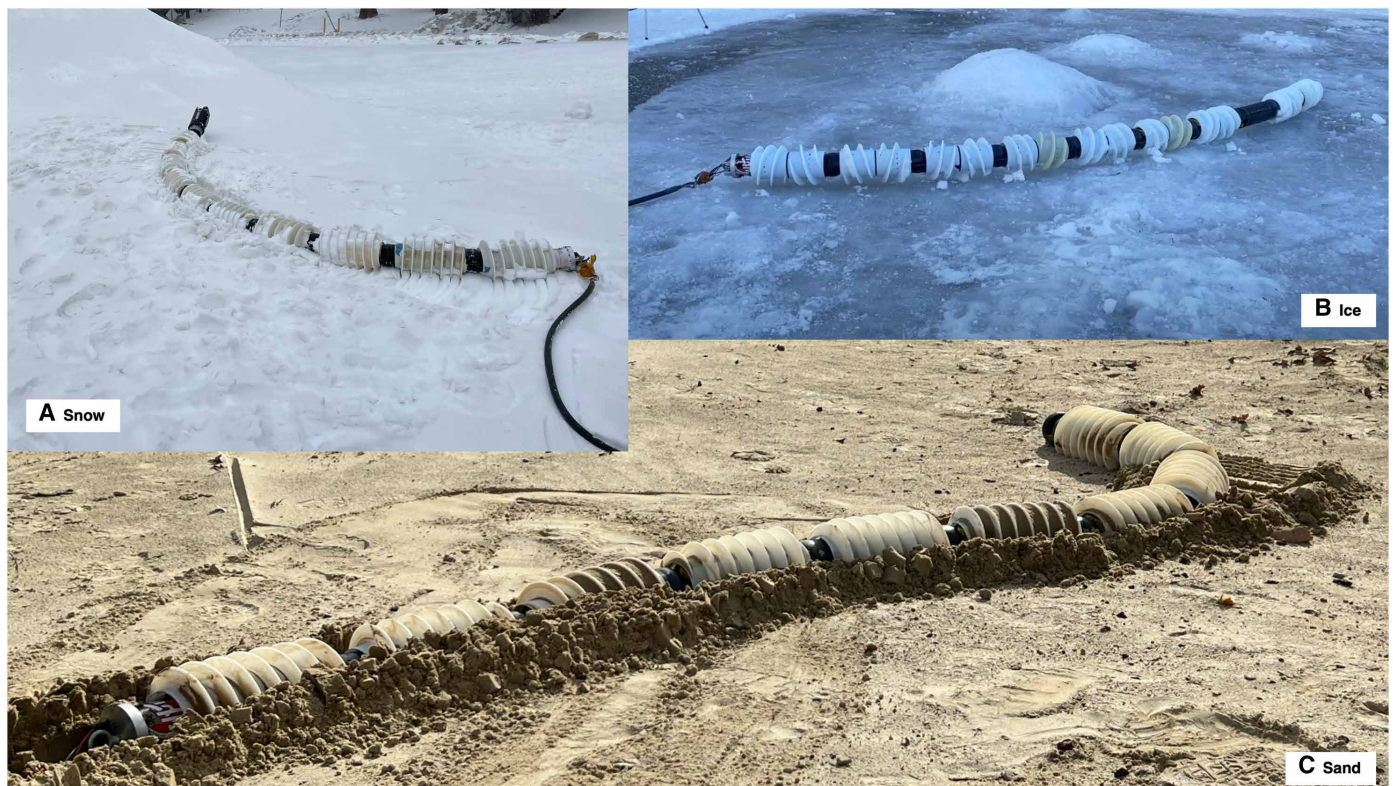
Fig. 6. Field test overview for surface scenarios. Robot tests in different environments: (A) consolidated and unconsolidated snow in Big Bear, California; (B) ice in JPL's Table Mountain facility; and (C) consolidated and unconsolidated sand at JPL's Mars Yard.
