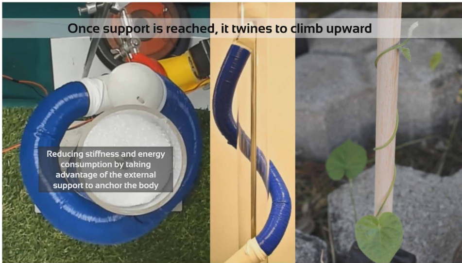
Movie 1. Overview of the principal climbing plant adaptive behaviors reached with the 3D printer-based growing robot for navigation in unstructured environments.
