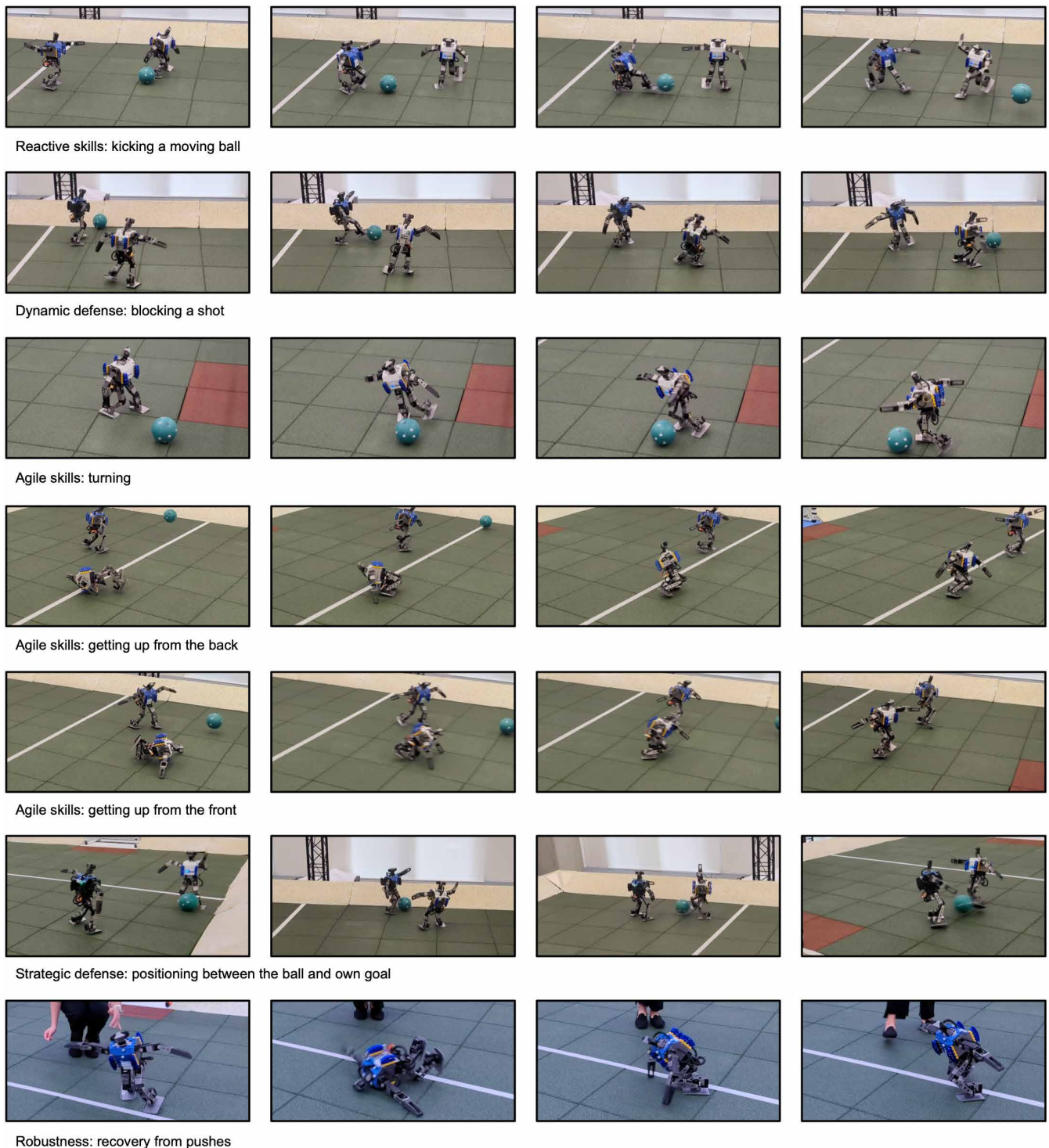
Fig. 3. Gallery of robot behaviors. Each row gives an example of a type of behavior that was observed when the trained policy was deployed on real robots. The top six rows are photographs taken from five consecutive matches played on the same day, using the same policy. The bottom row of photographs demonstrate the same policy but were not taken from match play.
