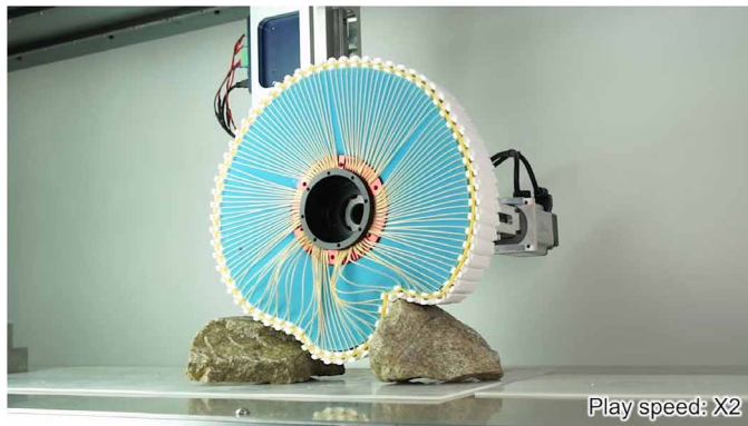
Movie 1. Demonstration of a vehicle with a variable-stiffness–morphing wheel. In a field demonstration, the mechanism realized stiffness variation based on variable surface tension.
