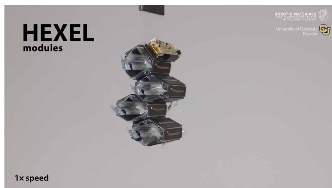
Movie 1. Working principle and demonstrations of HEXEL modules. HEXEL modules produce high-speed, high-strain actuation and serve as building blocks in rapidly reconfigurable robots that can be driven by untethered, snap-on driving electronics.
