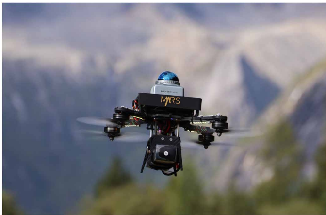
Movie 1. Overview of the proposed SUPER system. SUPER demonstrates its ability to safely navigate through unknown, cluttered environments at high speeds; avoid thin obstacles like power lines; and perform robustly in various scenarios, including object tracking and autonomous exploration.
