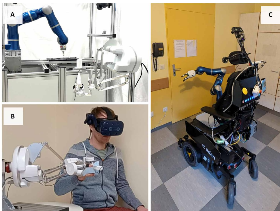
Fig. 8. Experimental hardware. (A) The DLR LWR at the back was under EPRC control and could be controlled via the lambda.7 input device. (B) The sigma.7 haptic input device was applied in the experiments on the ISS and in the elderly care facility. (C) The wheelchair-based robot EDAN was equipped with an eight-DoF robotic manipulator and a DLR CLASH hand.
