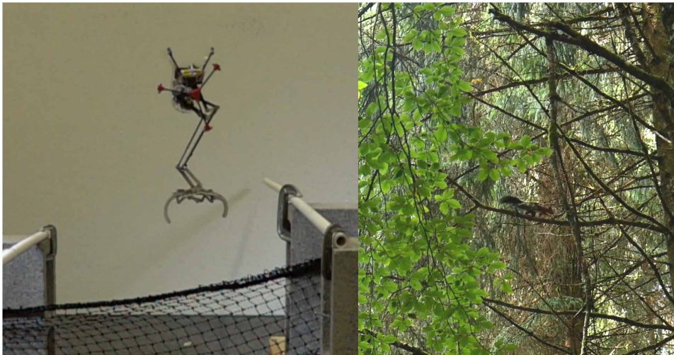
Movie 1. Overview of branch-to-branch leaping and balanced landing. This video presents robotic branch-to-branch leaps and balanced landings, demonstrated by the monopedal robot Salto.
