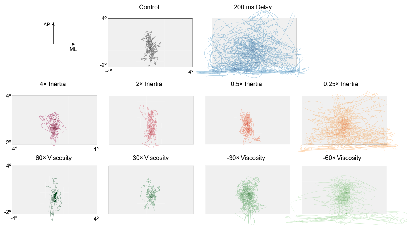
Fig. 2. CoM motion from all participants during balance trials (experiment 1). CoM motion from all participants ( n = 16 ) is depicted in the AP and ML directions for all control, delay, inertia, and viscosity trials. The gray shaded regions indicate the virtual limits ( 4^\circ anterior and mediolateral; 2^\circ posterior) within which the software of the robotic balance device simulated the inverted pendulum dynamics. CoM motion traces that are outside of the shaded regions indicate when participants exceeded the balance limits (considered virtual falls).
