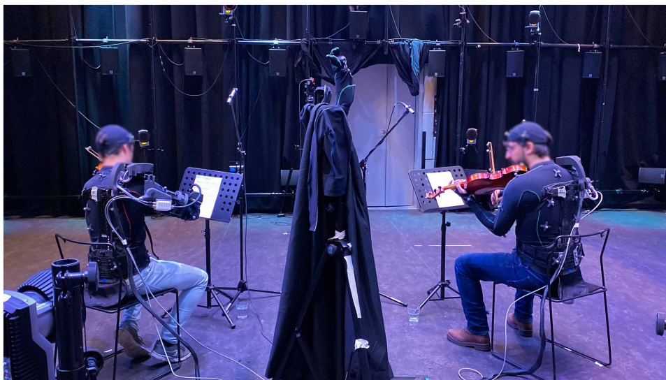
Movie 1. Summary of the study design and findings. This movie shows how exoskeletons can be used to create a virtual physical coupling between violinists, allowing them to feel each other's movements in real time. We show that this robot-mediated haptic feedback is more effective than traditional visual feedback in enhancing kinematic coordination and musical alignment.
